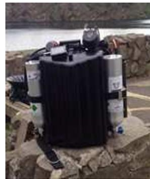
Apocalypse Type IV mCCR with AV1f PPO2 Dive Computer and Narked at 90 HUD, at Stoney Cove. The orange cable is from a Metalsub canister torch, located on the right side of the mCCR, strapped to the side-rail mounted 3L Oxygen cylinder.
