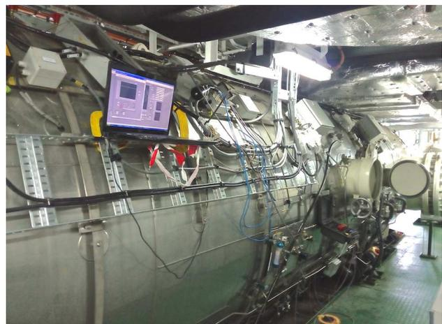
Above: Client's Sat complex under compliance test by Open Safety Aug 2017, using the Open Safety Respiratory Simulator. Our breathing simulators are available for purchase, or hire with supporting staff, onsite anywhere in the world.
